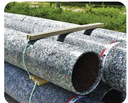
PVC pipe manufactured using material from recycled PVC.
