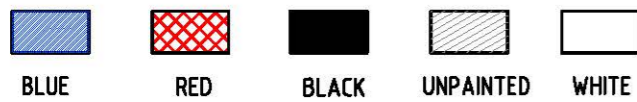
PAINTING COLOUR CODE FOR INDICATOR SIGNS NOTE : INSTALLER TO PAINT SIGN AND POST, IF PAINTING REQUIRED.
